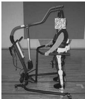
**Figure 1.** Patient performing gait training with the HAL exoskeleton.
