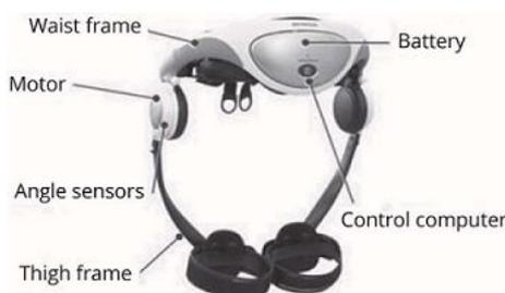
**Figure 3.** Honda Stride Management Assist (SMA) Device.
