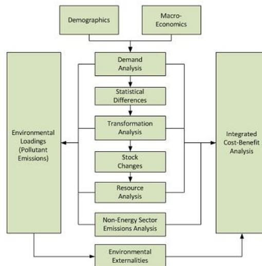
*Figure 2. Structure of LEAP model.*
