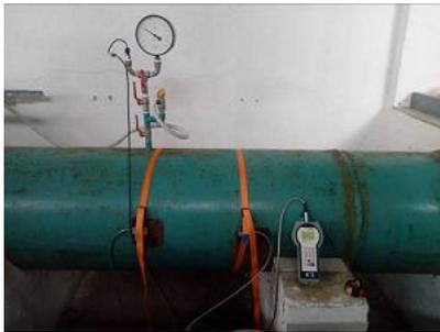
*a. measuring pressure and discharge.*
