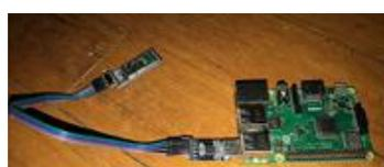
**Figure 7.** Interfacing Bluetooth module with Raspberry Pi3.
