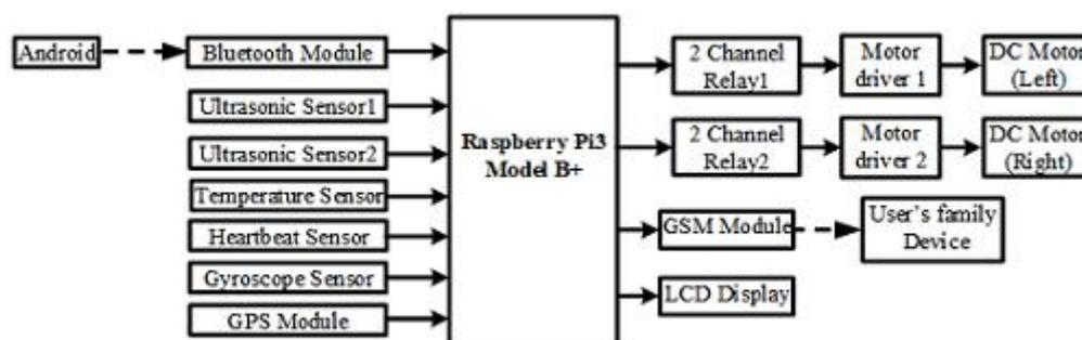
*Figure 1. Overall Block Diagram of the Proposed System.*
