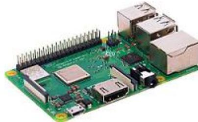
*Figure 2. Raspberry Pi 3 Model B+.*
