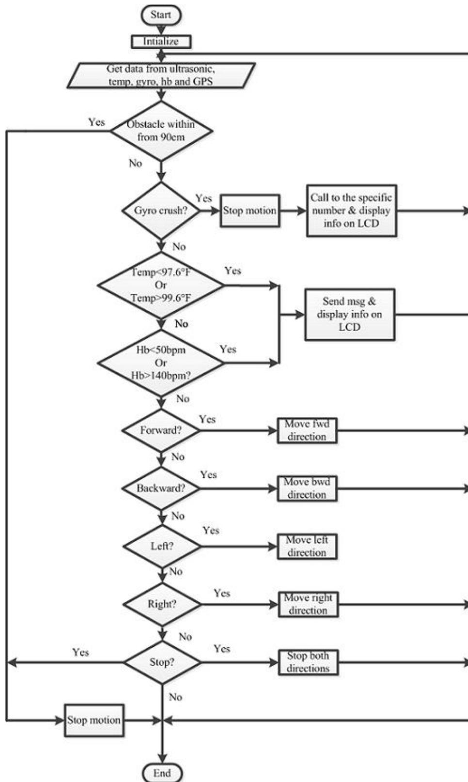
*Figure 5. The Flowchart of the Operation for the Motor Drive System.*
