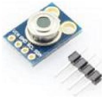
*Figure 3. Temperature Sensor (MLX90614).*
