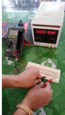
*Figure 10. Measuring the Voltage Divider.*
