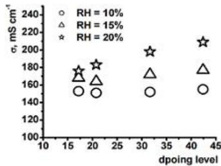
Figure 2. Effect of doping level on proton conductivity at different relative humidity [13].
