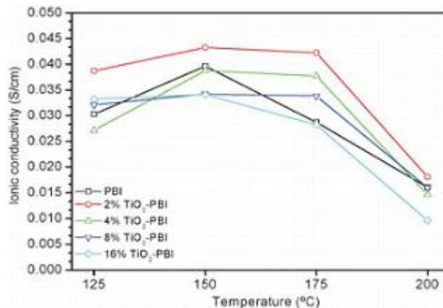
Figure 4. Ionic conductivity values of the TiO<sub>2</sub> composite membranes and the standard one at different temperatures. Acid bath = 75% wt [15].
