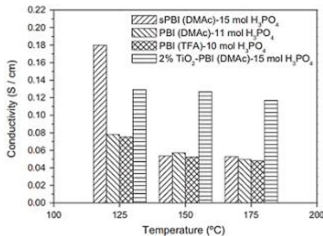
Figure 3. Proton conductivity for PBI membranes at different temperatures [14].
