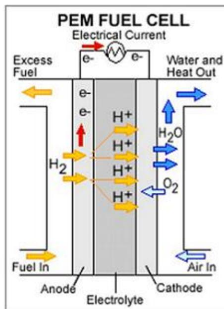
*Figure 1. The schematic principle of PEMFC-Reprinted from "Hydrogen Fuel Cells" by J. K. Harbeck, 2010, Stanford University.*
