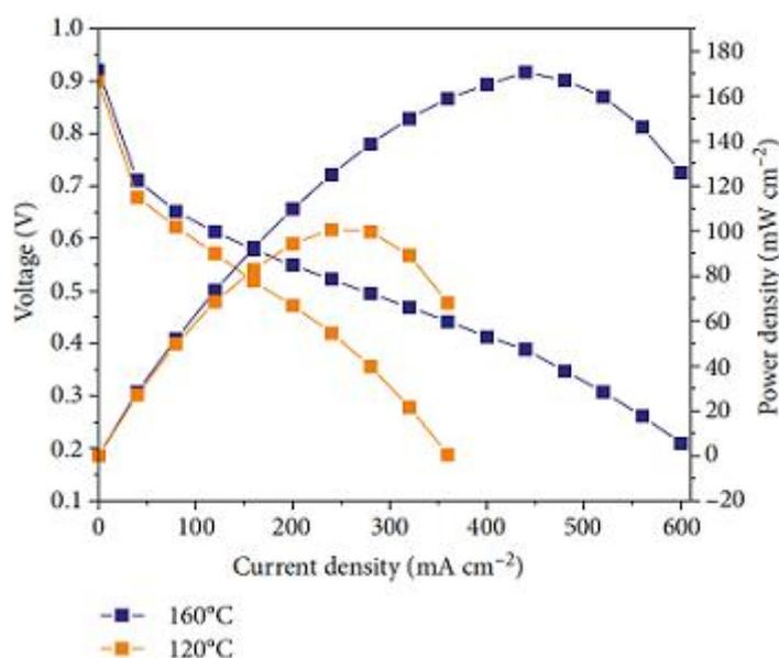
Figure 5. Single cell performance of PA-doped PEI-ER(1 : 2)/PBI at 120 °C and 160 °C [17].
