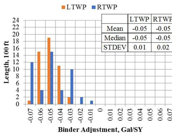
**Figure 2.** Distributions of Binder Rate Adjustment Output for 1 mile of Case III in the EB Direction.
