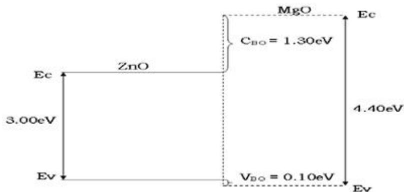
Figure 8. Band alignment in ZnO /MgO superlattice.
