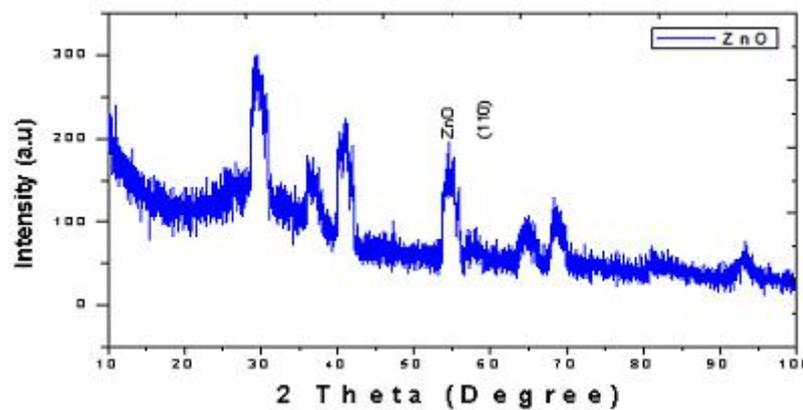
**Figure 3.** The XRD Pattern of ZnO.
