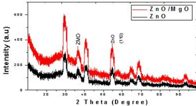
Figure 4. The XRD Pattern of ZnO and ZnO/MgO Superlattice.
