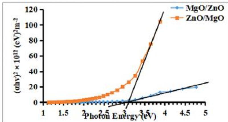
Figure 7. Plot of absorption coefficient squared versus photon energy for MgO/ZnO and ZnO/MgO superlattices.
