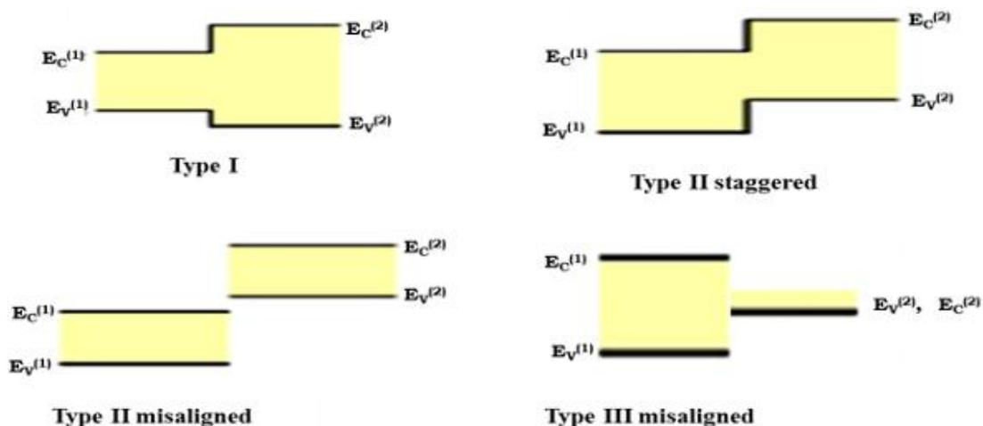
**Figure 2.** Types of Superlattice miniband structures.
