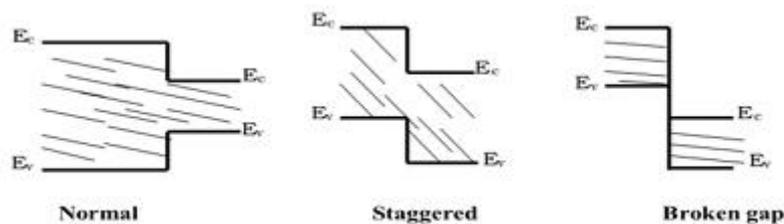
**Figure 1.** The relative alignment of the conduction and valence band edges.
