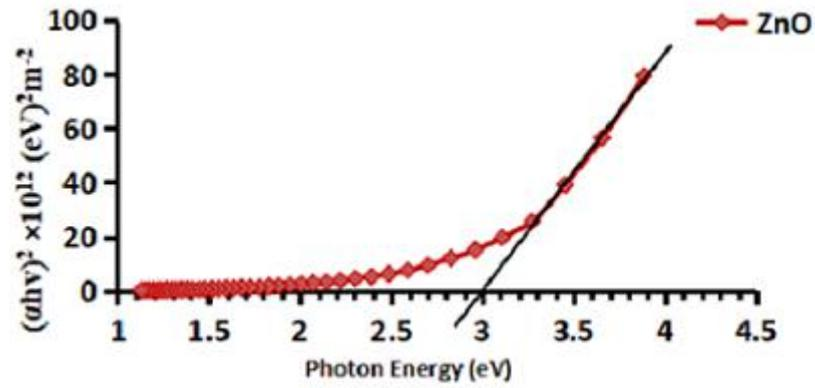
Figure 6. Plot of absorption coefficient squared versus photon energy for ZnO Thin film.
