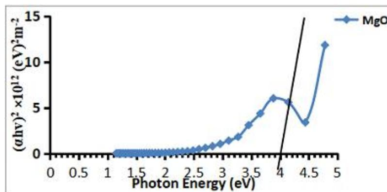
Figure 5. Plot of absorption coefficient squared versus photon energy for MgO Thin film.
