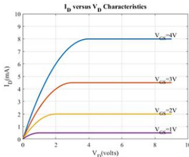
**Figure 1.** Voltage-Current Characteristics of Hybrid Materials-based MOSFET.
