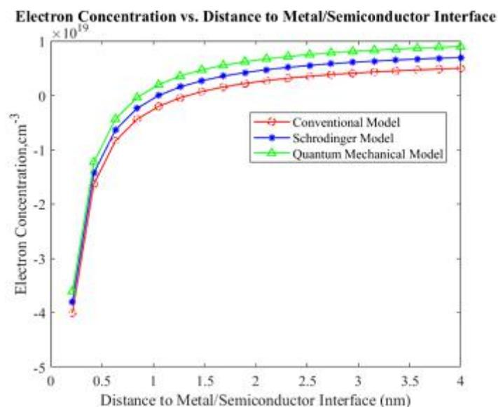
*Figure 3. Electron Concentration Vs Distance to Semiconductor Surface.*
