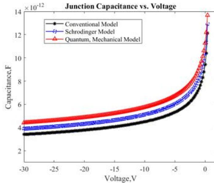
*Figure 2. Junction Capacitance Vs Voltage.*
