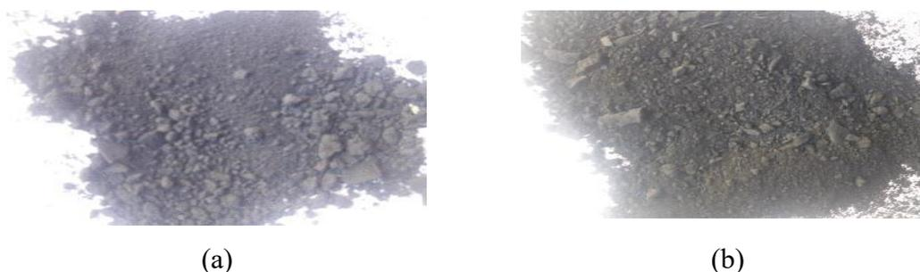
*Plate 1. Soot samples from (a) kerosene lamp and (b) kerosene stove.*
