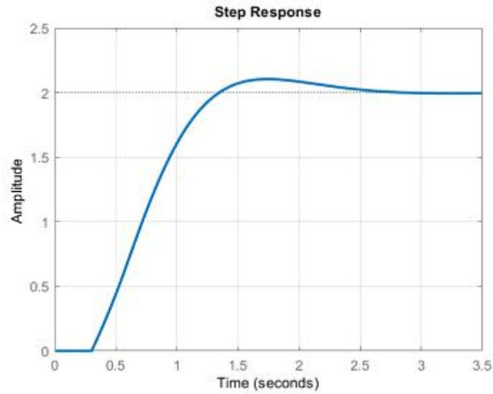
**Figure 3.** Step response of P Controller at  $L=0.3$ .
