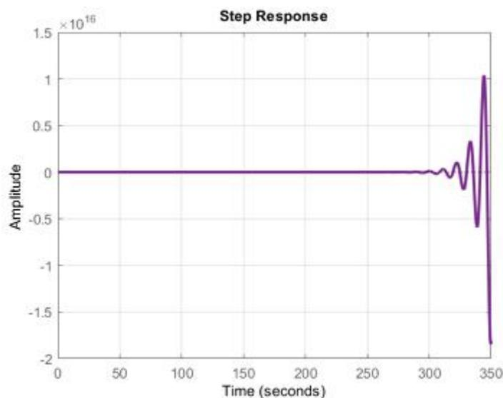
*Figure 9. Step response of PID Controller at  $L=1$ .*
