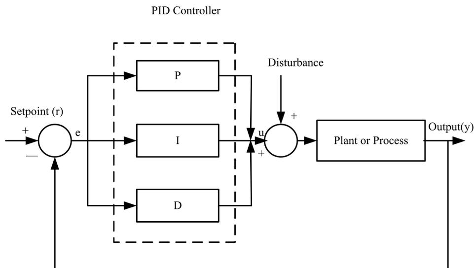
**Figure 1.** Block diagram of PID controller [6].
