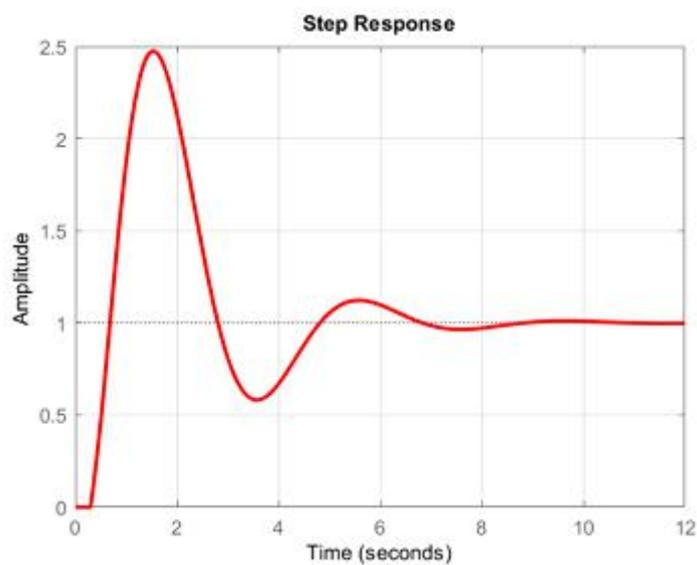
*Figure 5. Step response of PI Controller at  $L=0.3$ .*
