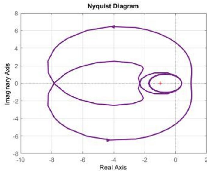
*Figure 8. Nyquist plot of PID Controller at  $L=1$ .*
