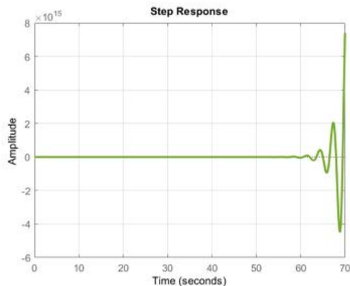
*Figure 7. Step response of PD Controller at  $L=1$ .*
