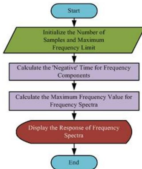
**Figure 5.** Flowchart of Implementation for Frequency Spectra.
