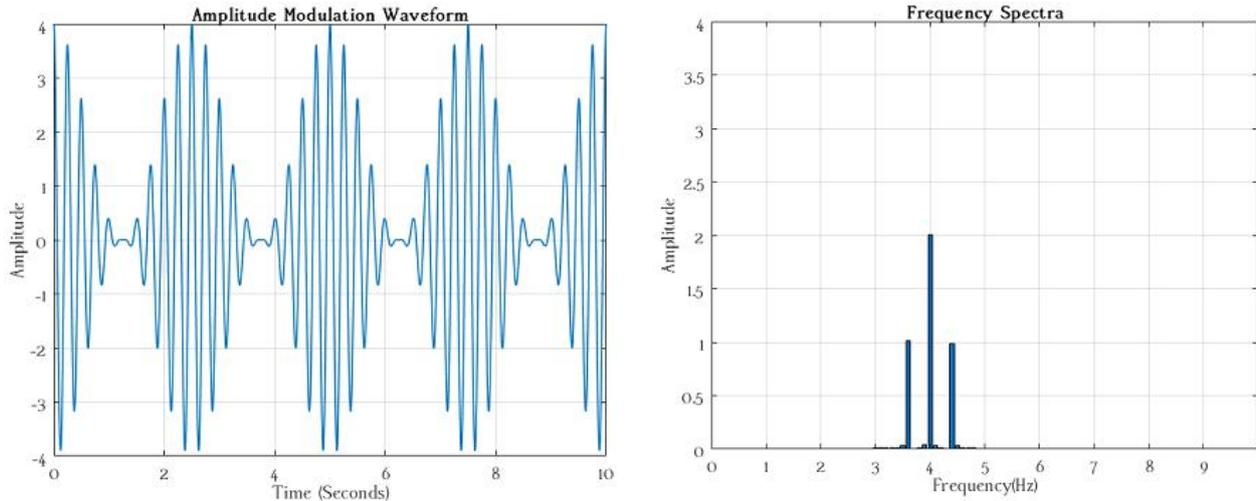
**Figure 11.** (a) Amplitude Modulation Waveform ( $A_c = 2.0, f_c = 4.0, A_m = 2.0, f_m = 0.4, \mu = 1.0$ ),
