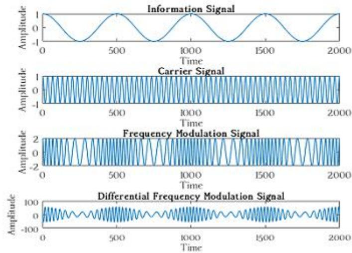
**Figure 13.** Frequency Modulation Signal ( $f_c = 3$ ,  $f_m = 0.2$ ,  $A_m = 1$ ,  $A = 2$ ,  $k_f = 10$ ).
