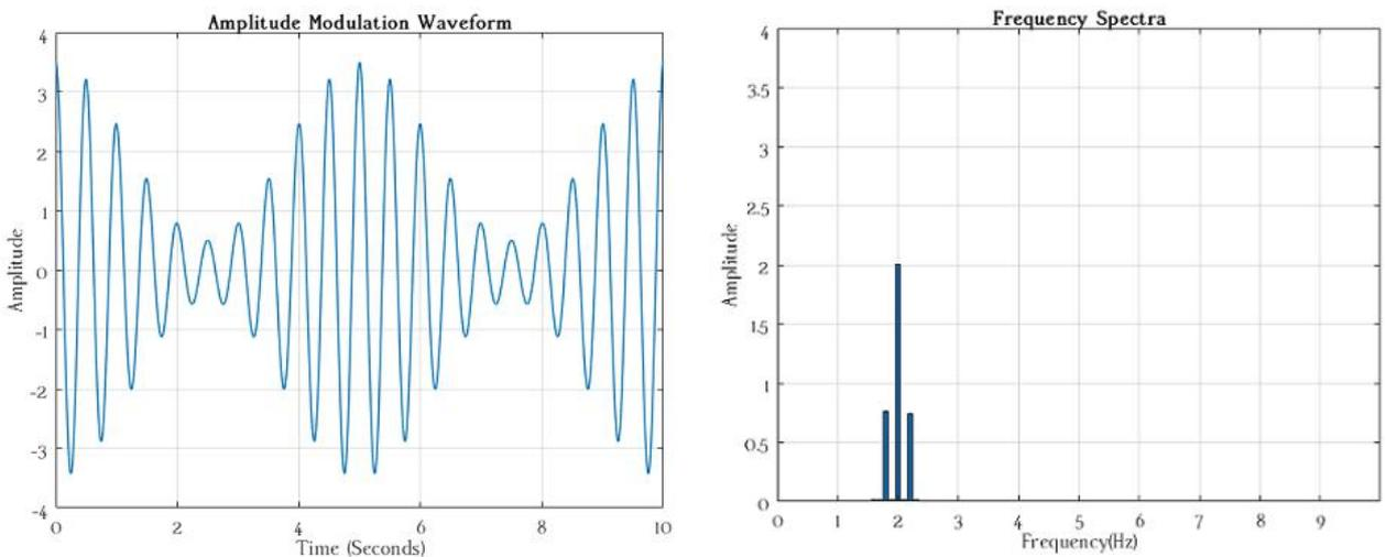
**Figure 10.** (a) Amplitude Modulation Waveform ( $A_c = 2.0$ ,  $f_c = 2.0$ ,  $A_m = 1.5$ ,  $f_m = 0.2$ ,  $\mu = 0.75$ ),
