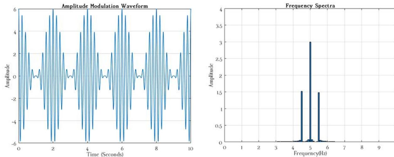
**Figure 12.** (a) Amplitude Modulation Waveform ( $A_c = 3.0, f_c = 5.0, A_m = 3.0, f_m = 0.5, \mu = 1.0$ ),
