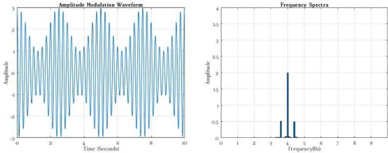
**Figure 8.** (a) Amplitude Modulation Waveform ( $A_c = 2.0$ ,  $f_c = 4.0$ ,  $A_m = 1.0$ ,  $f_m = 0.4$ ,  $\mu = 0.50$ ),
