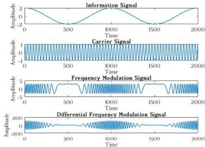
**Figure 16.** Frequency Modulation Signal ( $f_c = 3$ ,  $f_m = 0.1$ ,  $A_m = 2.0$ ,  $A = 3$ ,  $k_f = 10$ ).
