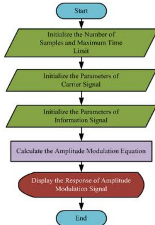
**Figure 4.** Flowchart of Implementation for Amplitude Modulation Signal.
