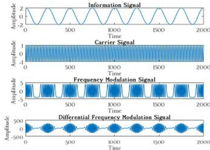
**Figure 14.** Frequency Modulation Signal ( $f_c = 6$ ,  $f_m = 0.4$ ,  $A_m = 2$ ,  $A = 4$ ,  $k_f = 20$ ).
