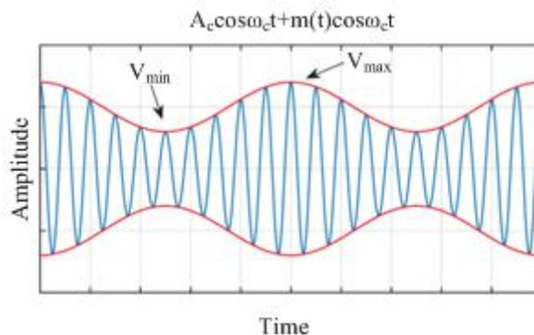
**Figure 1.** Standard Amplitude Modulation Waveform.
