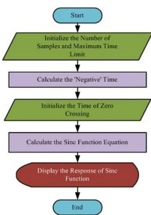
**Figure 3.** Flowchart of Implementation for Sinc Function in MATLAB Environments.
