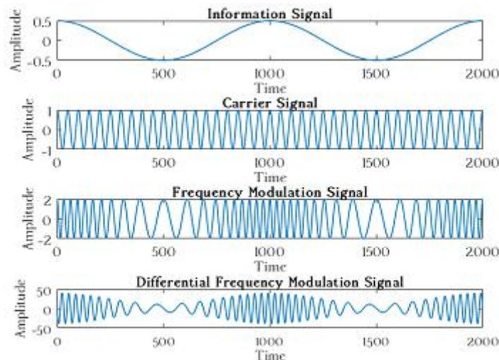
**Figure 15.** Frequency Modulation Signal ( $f_c = 2$ ,  $f_m = 0.1$ ,  $A_m = 0.5$ ,  $A = 2$ ,  $k_f = 15$ ).
