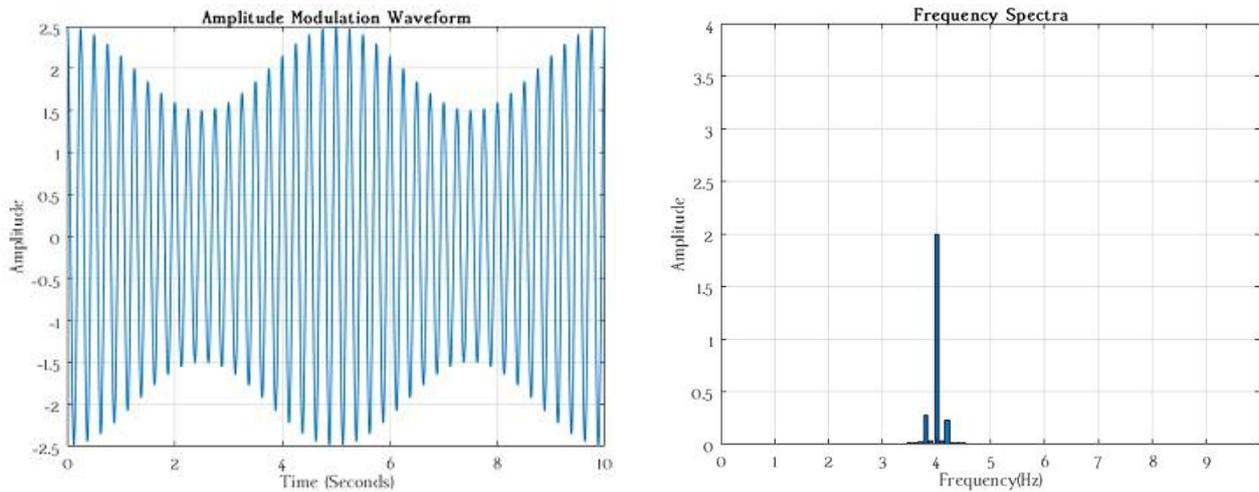
**Figure 9.** (a) Amplitude Modulation Waveform ( $A_c = 2.0$ ,  $f_c = 4.0$ ,  $A_m = 0.5$ ,  $f_m = 0.2$ ,  $\mu = 0.25$ ),
