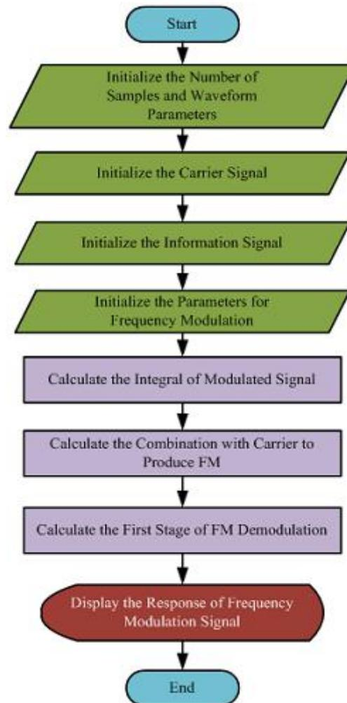
*Figure 6. Flowchart of Implementation for Frequency Modulation Signal.*
