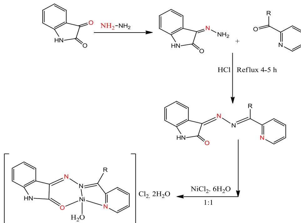
**Figure 14.** Synthesis route of Schiff base and Ni complex.
