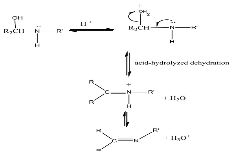
**Figure 1.** General Scheme for the preparation of Schiff bases.
