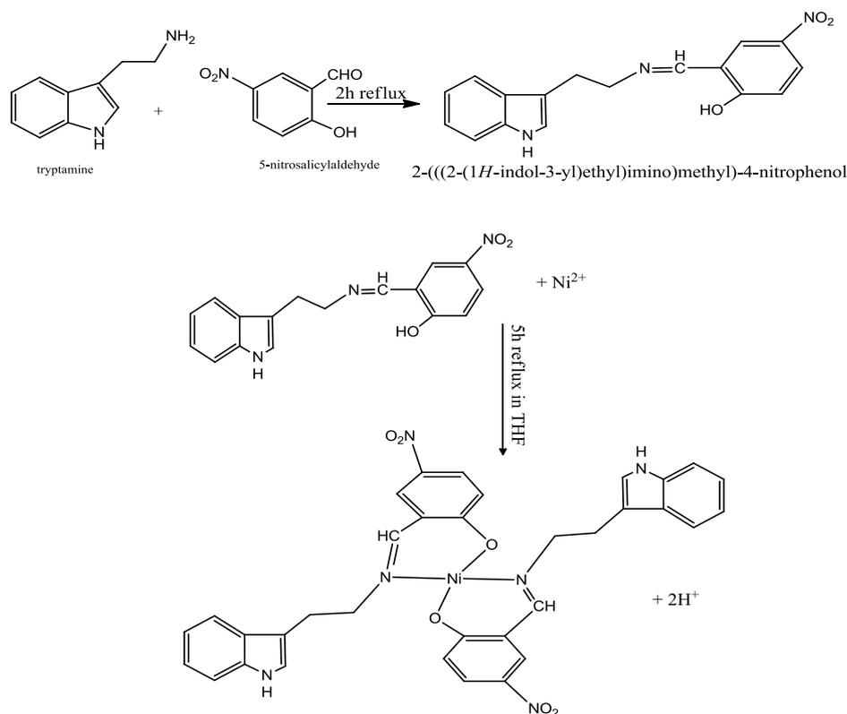
**Figure 11.** Synthesis route of Schiff base ligand and its Ni complexes.
