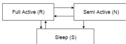
*Figure 1. The sensor node status change diagram.*
