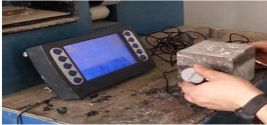
*Figure 4. Ultrasonic wave test process.*
