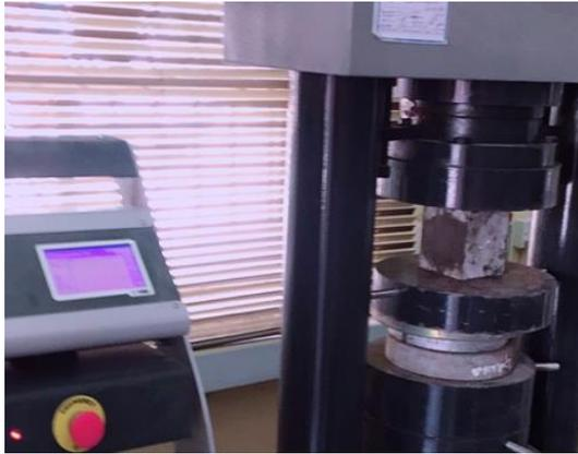
**Figure 6.** Compressive strength test.
