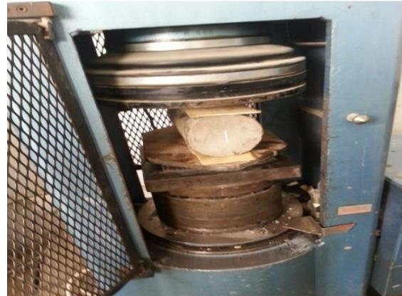
**Figure 7.** Indirect Tensile strength test.
