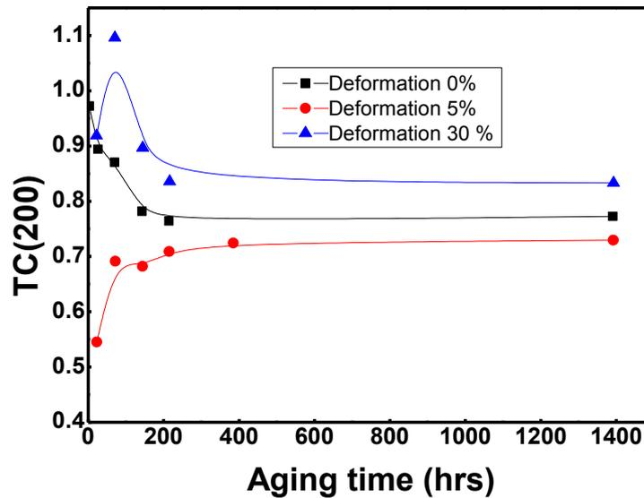
Figure 9. The texture coefficient at (200) vs. ageing time.
