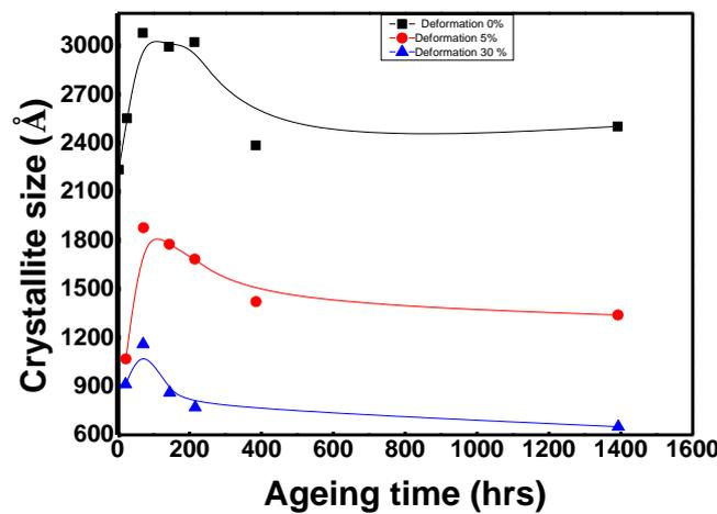
Figure 4. Crystallite size vs. aging time.
