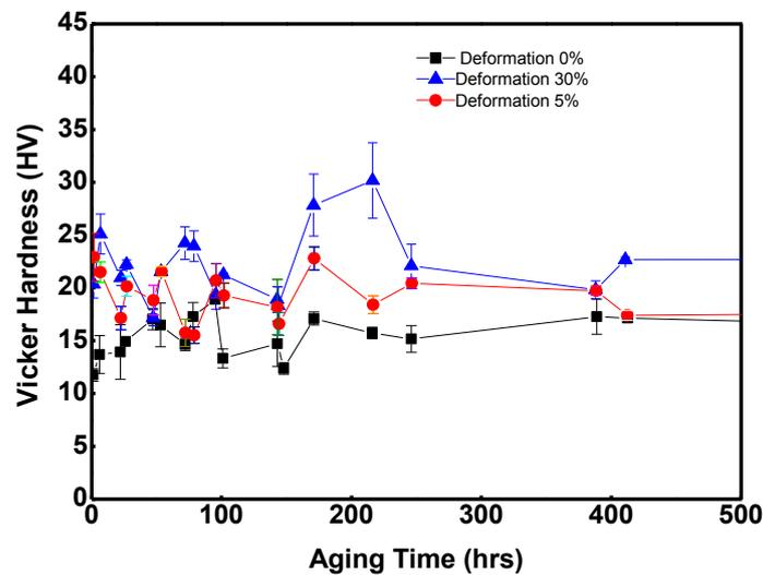
Figure 2. The Vickers hardness vs. aging time.
