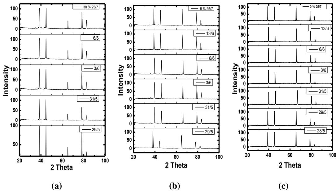
Figure 3. XRD patterns for different 6063 Al-ally samples at (a) non-deformed, (b) 5 % and (c) 30 % degree of deformation.
