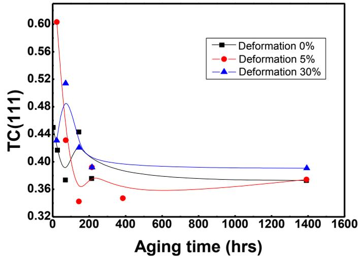
Figure 8. The texture coefficient at (111) vs. ageing time.
