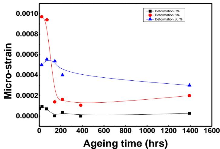
Figure 5. Micro-strain vs. aging time.
