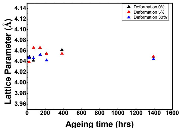
Figure 6. Lattice parameter vs. aging time
