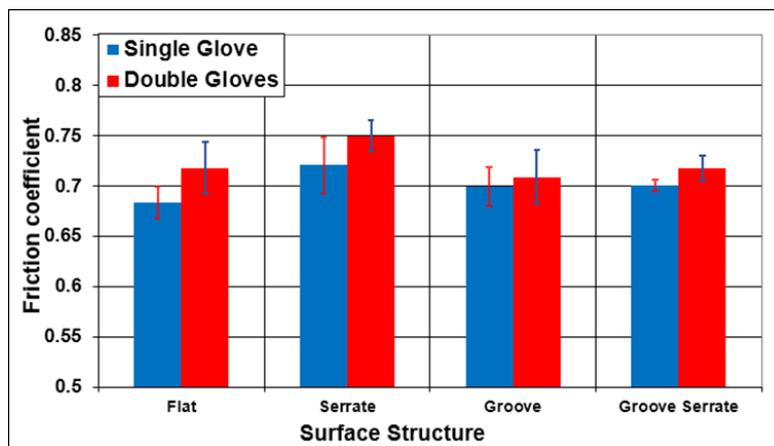
Figure 6. Static friction coefficients for single and double gloves in case of wet condition.
