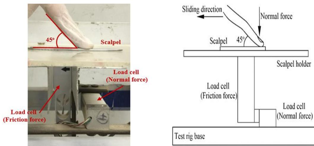
**Figure 2.** The test rig and a schematic of the friction measurement process.
