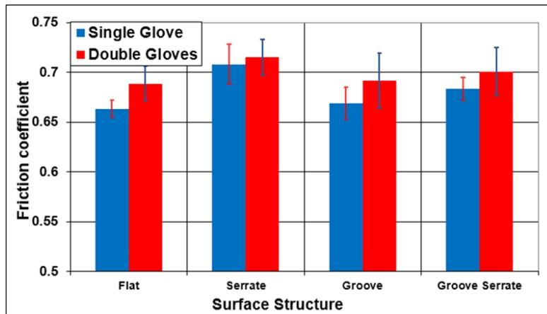
Figure 5. Static friction coefficients for single and double gloves in case of the dry condition.
