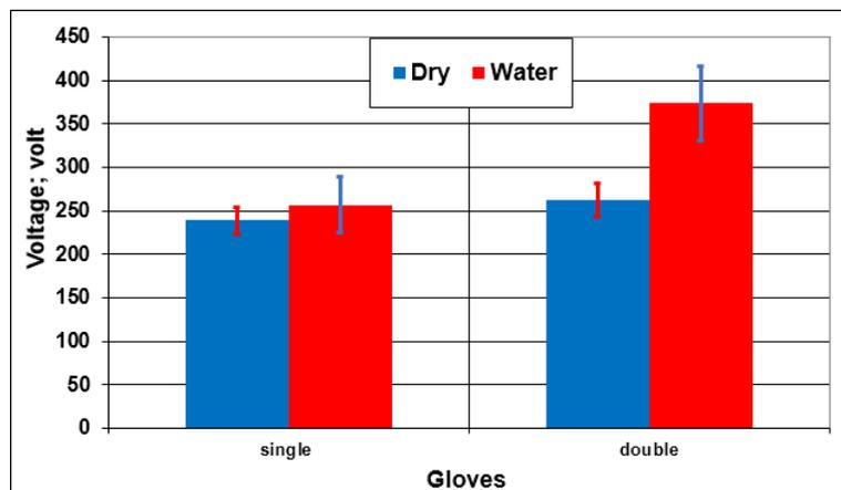
Figure 7. Electrostatic charge generated on the scalpel surface during single and double gloves sliding in dry and wet conditions.
