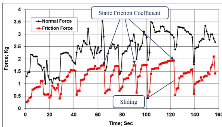
Figure 3. Data from the normal and friction force load cells.
