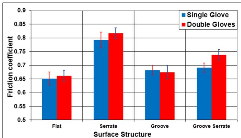
*Figure 9. Static friction coefficients for single and double gloves in case of blood mixed water condition.*
