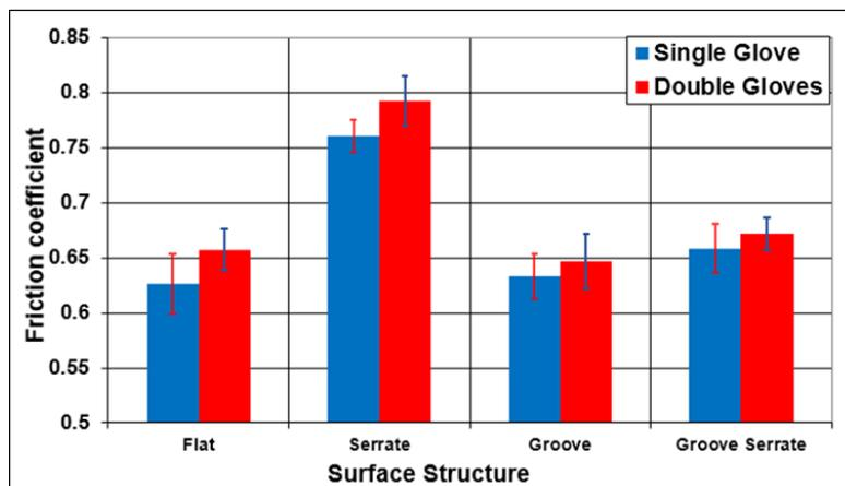
*Figure 8. Static friction coefficients for single and double gloves in case of a blood condition.*
