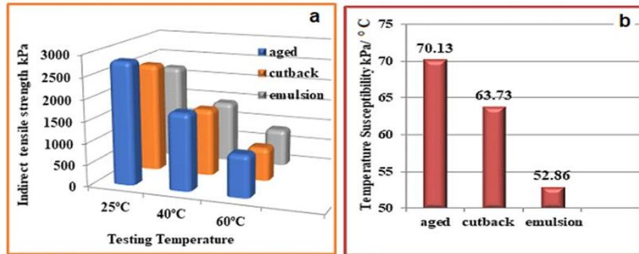
Figure 5. (ITS) and Temperature Susceptibility for Aged and Recycled Mixtures.
