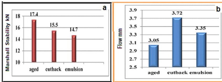
**Figure 4.** Variation of Marshal Stability and flow for Aged and Recycled Mixture.
