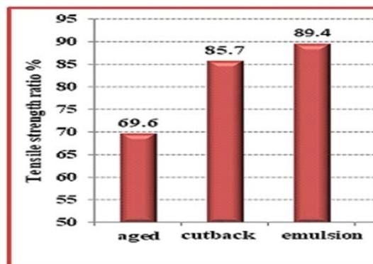
Figure 6. Tensile Strength Ratio for Aged and Recycled Mixtures.
