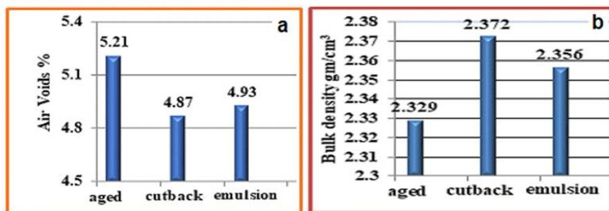
Figure 3. Variation of air voids and bulk density for Aged and Recycled Mixture.
