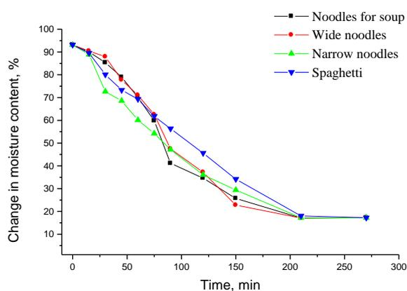
**Figure 2.** Changing the moisture content of pasta on 55 °C.
