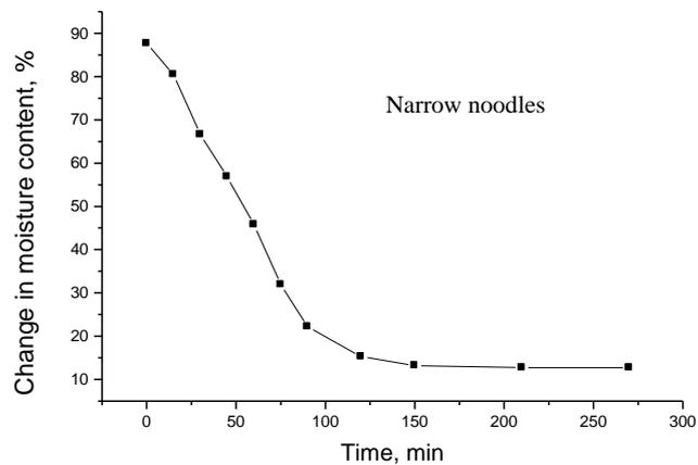
*Figure 9. Exponential value of change of moisture content with time for narrow noodles.*
