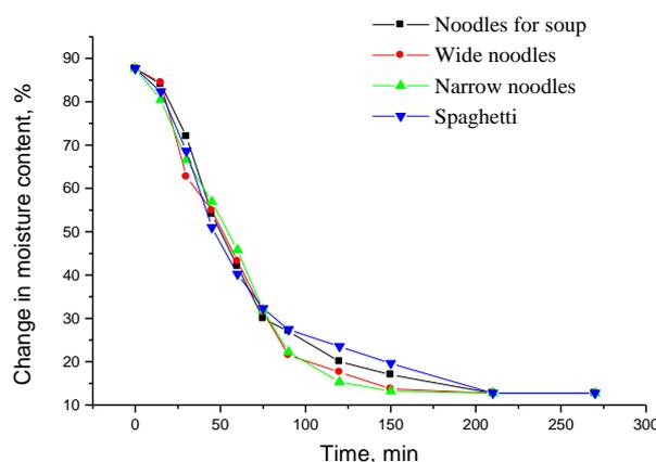
**Figure 6.** Changing the moisture content of pasta on 80 °C.
