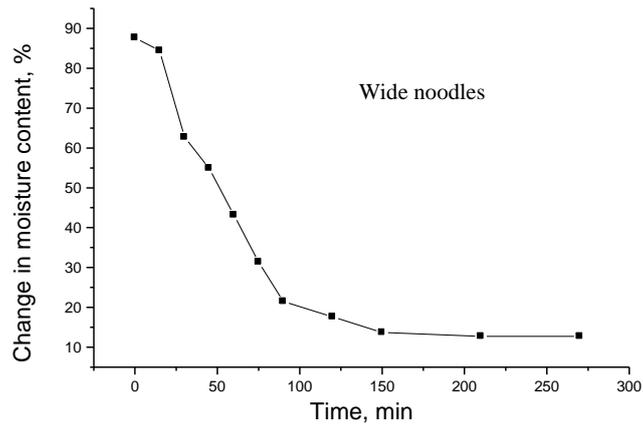
*Figure 8. Exponential value of change of moisture content with time for wide noodles.*
