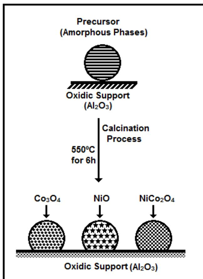
Figure 3. Schematic representation of phase changes during calcination process.
