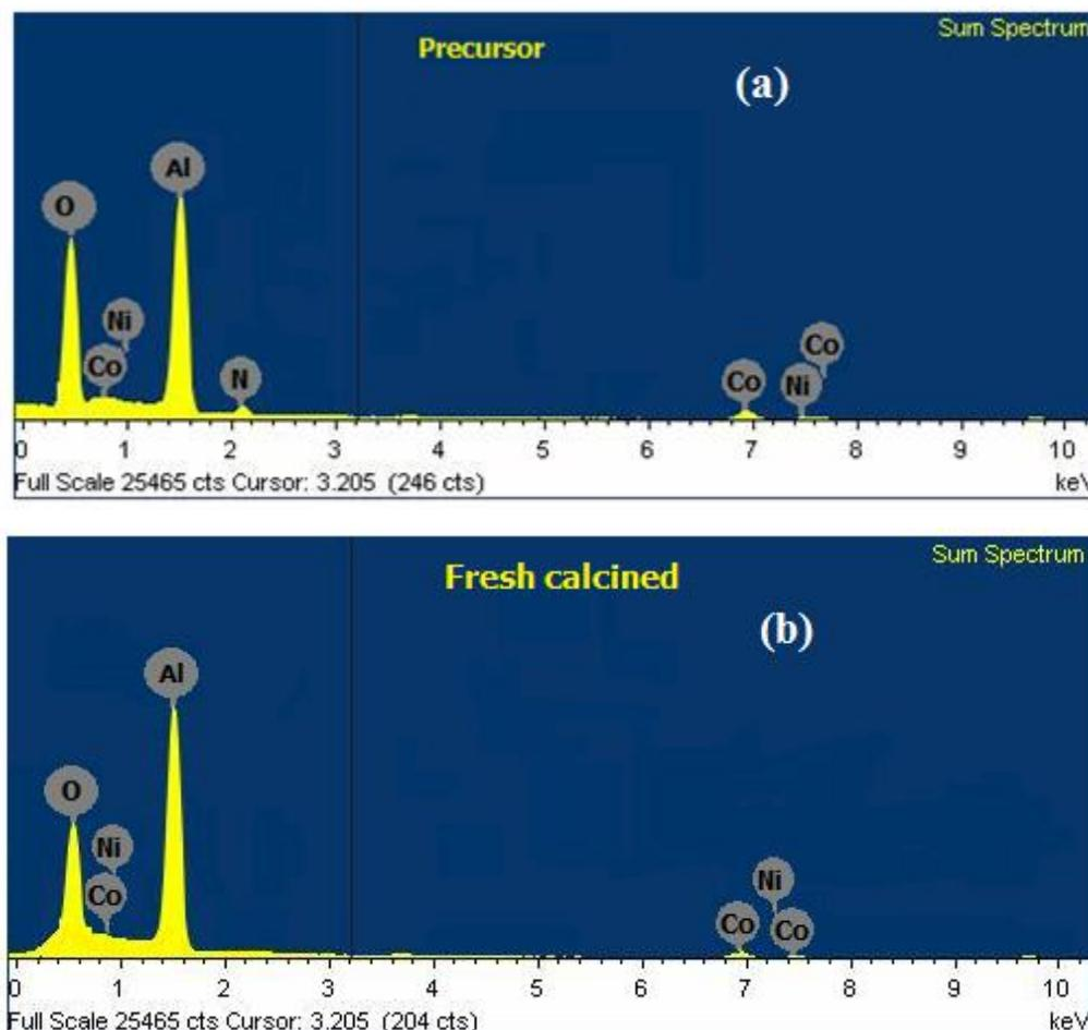
**Figure 5.** EDS spectrums of Co-Ni/Al<sub>2</sub>O<sub>3</sub> catalyst in (a) precursor and (b) calcined catalyst.
