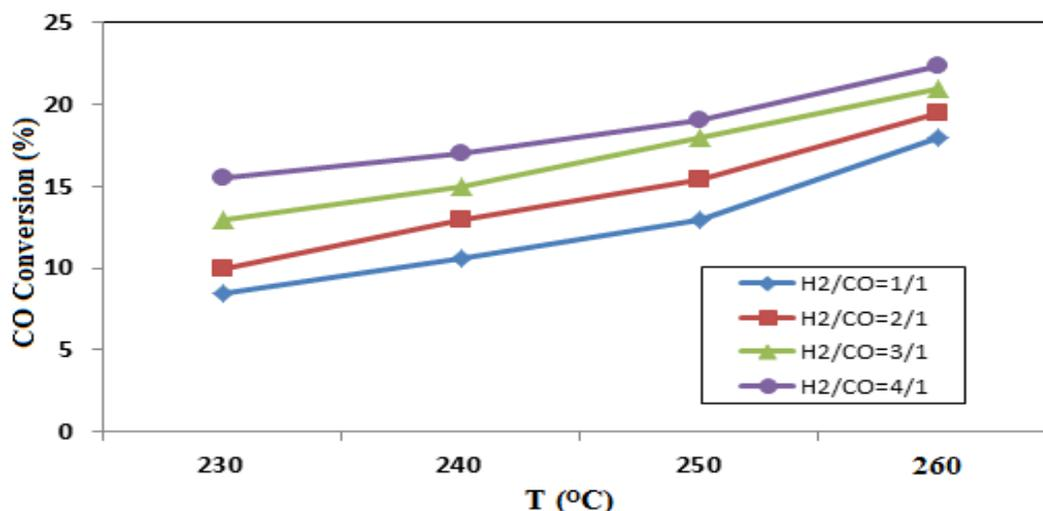
**Figure 6.** Effect of H<sub>2</sub>/CO feed ratio on the CO conversion at different temperatures (230-260 °C).
