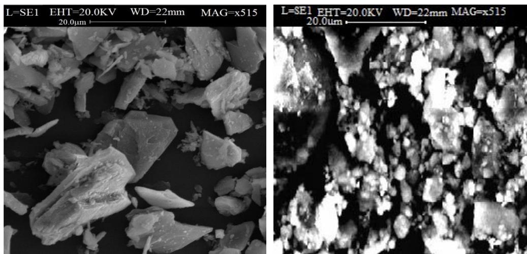
**Figure 4.** SEM images of Co-Ni/Al<sub>2</sub>O<sub>3</sub> catalyst in (a) precursor and (b) calcined catalyst.
