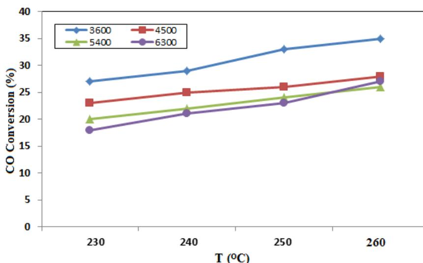
**Figure 8.** Effect of GHSV on the CO conversion at different temperatures (230-260 °C).
