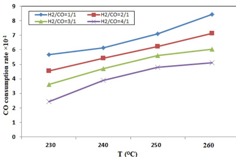
**Figure 7.** Effect of H<sub>2</sub>/CO feed ratio on the CO consumption rate at different temperatures (230-260 °C).
