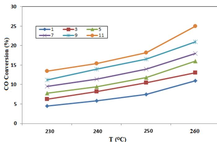
**Figure 10.** Effect of reaction pressure on the CO conversion at different temperatures (230-260 °C).
