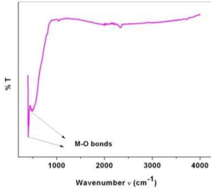
**Figure 3.** FTIR spectrum of ZnTiO<sub>3</sub> ceramic.
