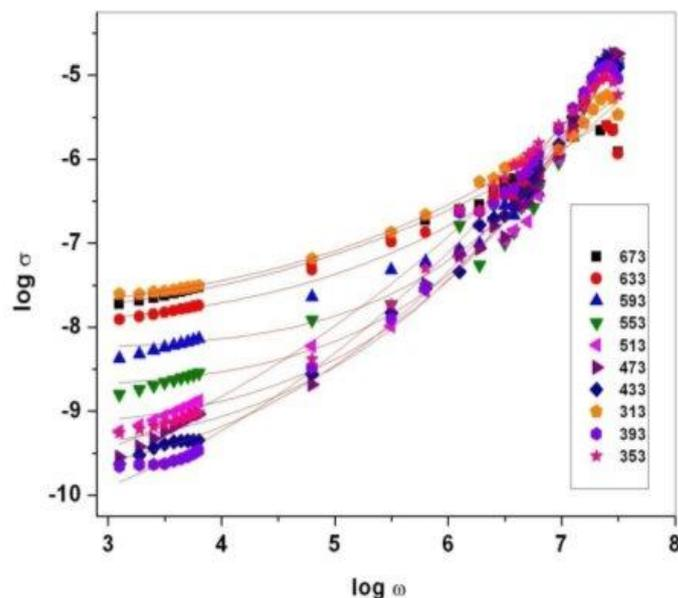
Figure 9. The  $\log \sigma$  versus frequency plots of  $\text{ZnTiO}_3$  ceramic.
