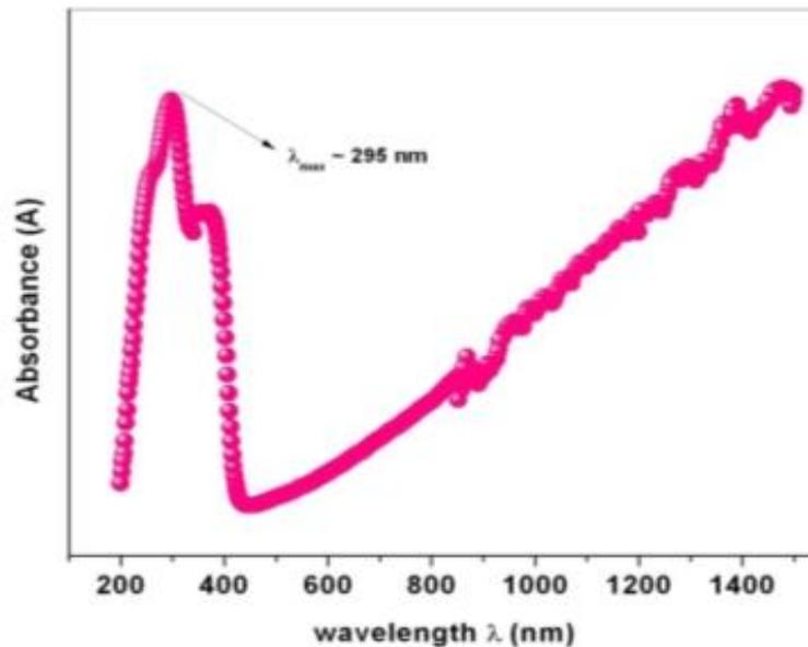
**Figure 4.** The absorption spectrum of ZnTiO<sub>3</sub> ceramic.
