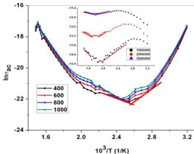
**Figure 8.** The  $\ln \sigma_{ac}$  and  $1000/T$  plots of  $\text{ZnTiO}_3$  ceramic.
