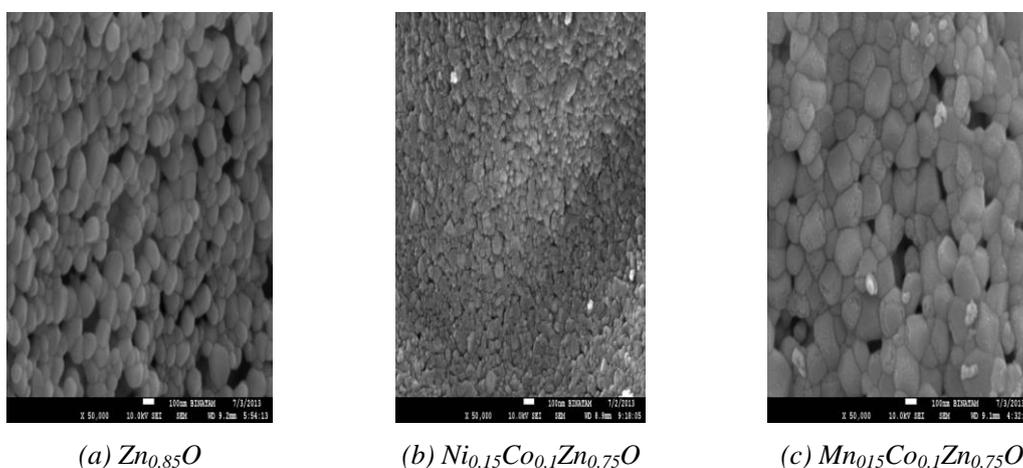
Figure 2. Field emission scanning electron micro-graphs (FE-SEM) of  $TM_{0.15}Co_{0.1}Zn_{0.75}O$  Nanoparticles.
