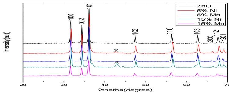
Figure 1. XRD patterns for  $TM_xCo_{0.1}Zn_{0.9-x}O$ .
