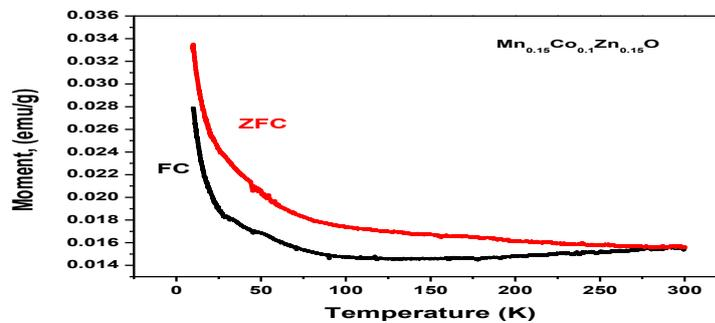
Figure 5(b). Zero Field Cooling (ZFC) and Field Cooling (FC) at room temperature for  $Mn_{0.15}Co_{0.1}Zn_{0.75}O$  Nanoparticles.
