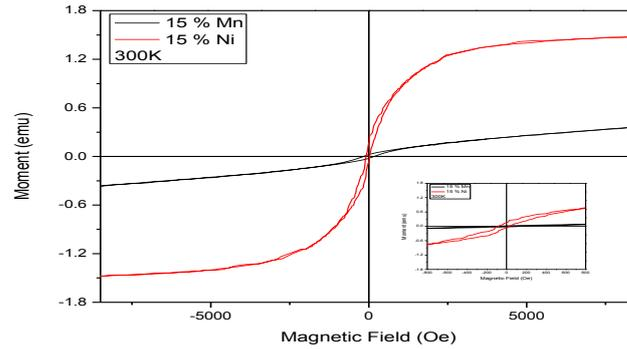
Figure 4. *M–H* curve of  $TM_{0.15}Co_{0.1}Zn_{0.75}O$  Nanoparticles for both samples.
