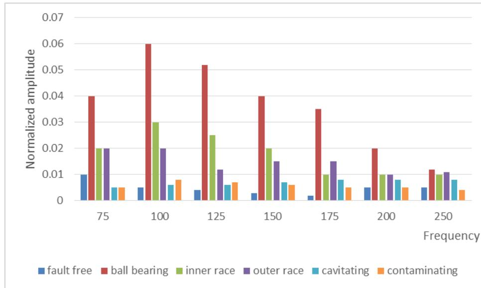
Figure 9. Frequency spectrum of motors at frequency selection.
