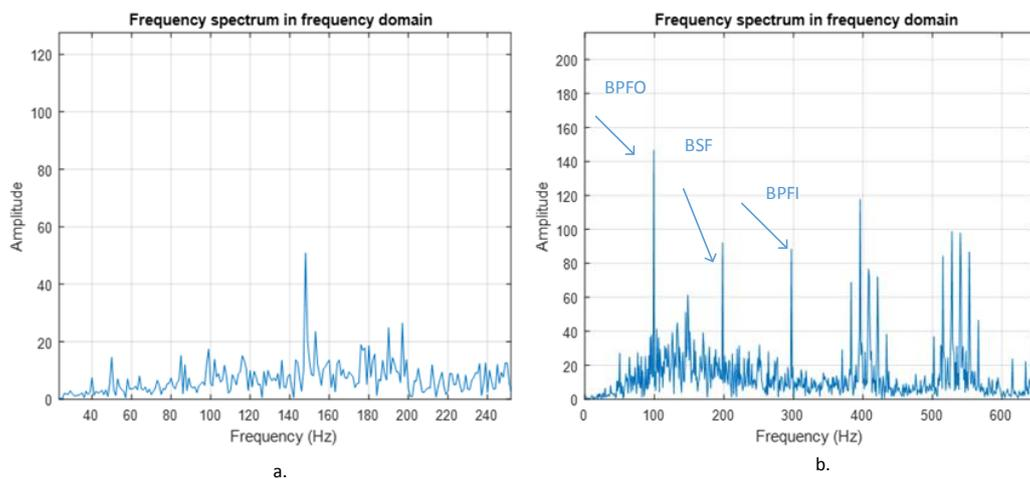
Figure 10. Demodulation with STFT result after preprocessing for a. healthy, b. ball bearing fault.
