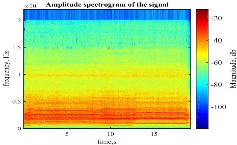
**Figure 5.** Spectrogram of healthy motor.
