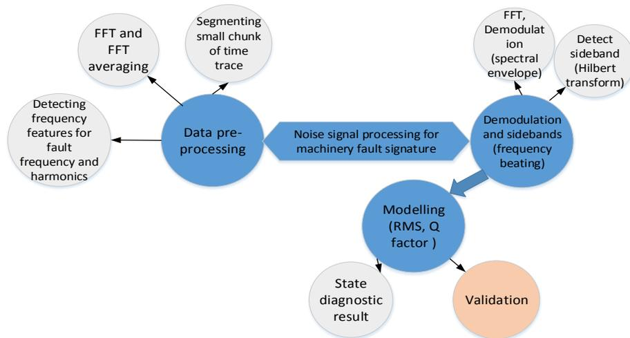
Figure 3. Automated noise signal processing scheme.
