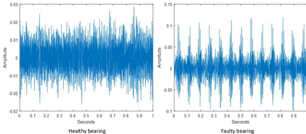
**Figure 8.** Pre-processed noise signal in time domain.
