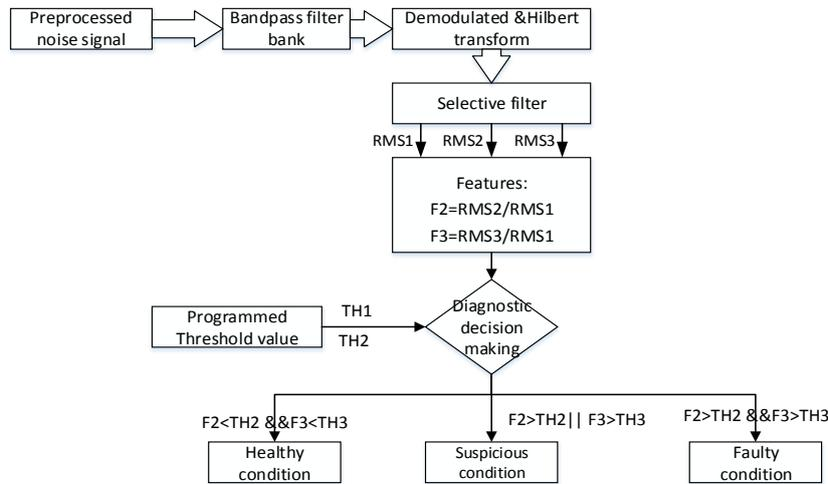
**Figure 7.** Flowchart of decision making for fault detection.
