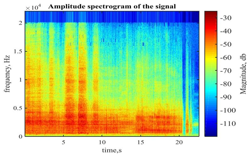
**Figure 6.** Spectrogram of motor with gear tooth defects.
