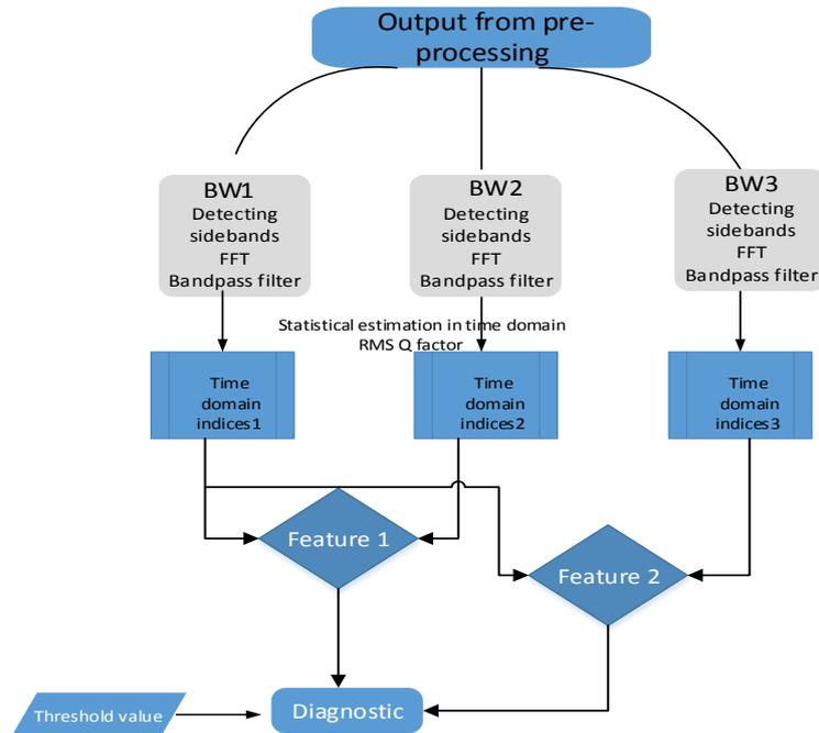
Figure 11. Automated fault detection algorithm.
